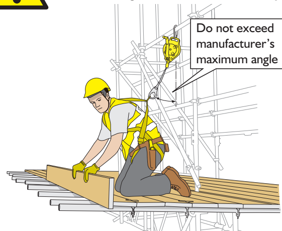
Figure 82: Falling object protection fan erected using a retrievable inertia reel.
