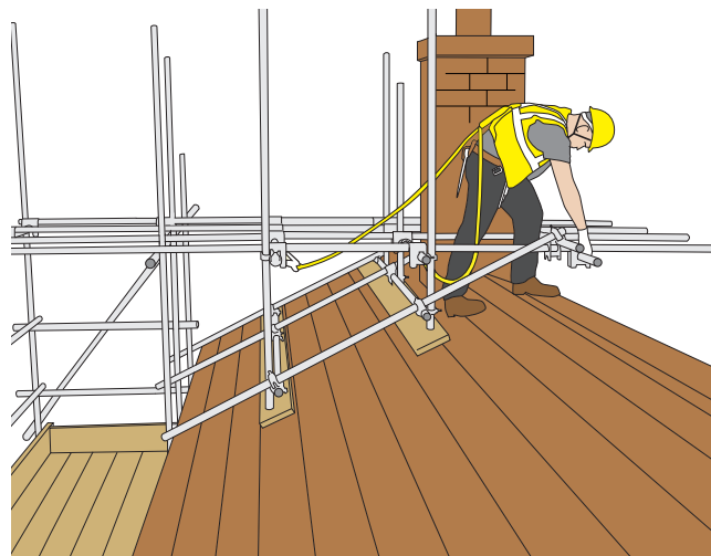
Figure 79: Example of a roof saddle sequence of work with eaves edge protection and continual attachment maintained using a double lanyard system of work.
