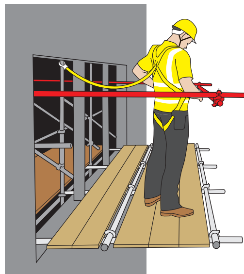
(iii) Needles (extended transoms) are boarded out to create a scaffolders' safe zone to complete the truss-out scaffold.
