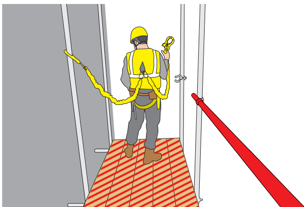
Figure 49: Double lanyard system using two separate fall arrest lanyards.
