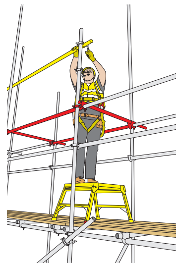
Figure 72: An example of an anchor point for a proprietary scaffolding system as per the manufacturers' instructions.
