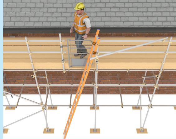
Example of a self-closing ladder safety gate.
