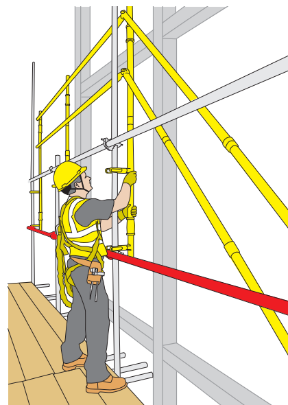
Figure 31: Shows the modified sequence of erection to allow an AGS to be used on the inside face before fixing transoms, ties or inside board brackets above.
