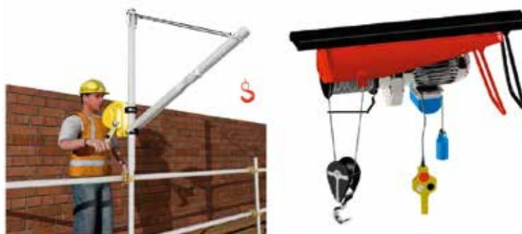
Wherever a jib crane is used to lift loads greater than 50 kg, consideration should be given to the need for the scaffold to be strengthened at the location of the crane and additional or stronger ties to the building provided, following guidance from the manufacturer or from a scaffolding designer.
