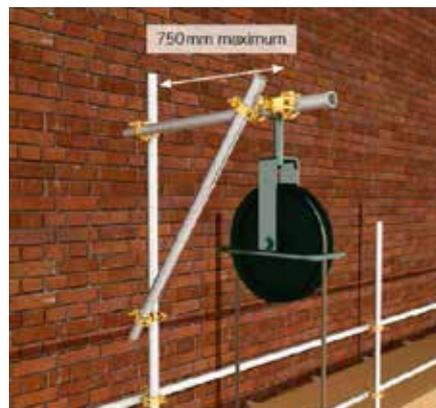
Alternatively, a vertical tube may be fixed near to the wall to form a puncheon, connected to the putlogs at two working levels with right-angled couplers. This puncheon should extend upward to connect to the horizontal tube, forming a supporting structure similar to the one for an independent scaffold.
