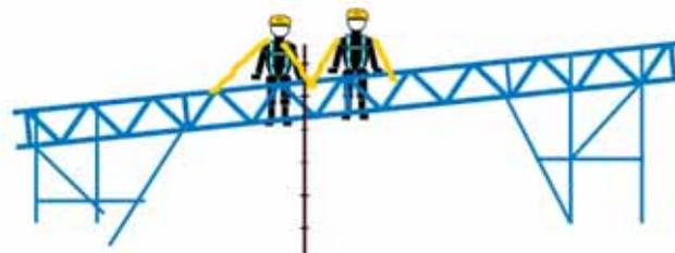
*Alternatively, a metal ladder can be lowered into position and secured in position (fixed with single clips and doubles on top, possibly with a tube fixed through under the metal rung), prior to instructing the fallen operative to ascend the secured ladder and move to a place of safety, before the removal of the lanyard, as detailed above).*
