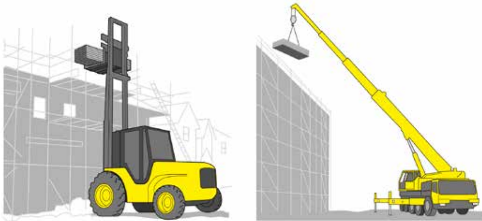
Figure 4 – Examples of site mechanical handling equipment utilised for scaffolding.
