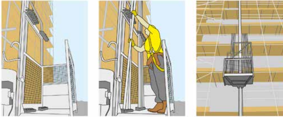
Figure 2 – Examples of goods hoists adapted for scaffold materials.
