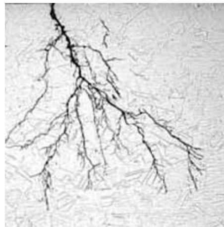
Figure 2 (Microstructure of Metal Displaying SCC)
