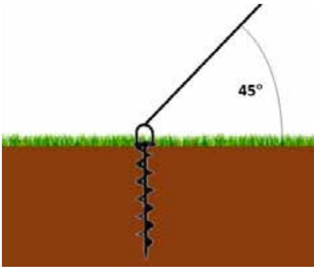
Figure 4 Helical Anchor (Spiral type)
