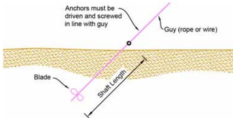
Figure 3 Helical Anchor (Single helix type)
