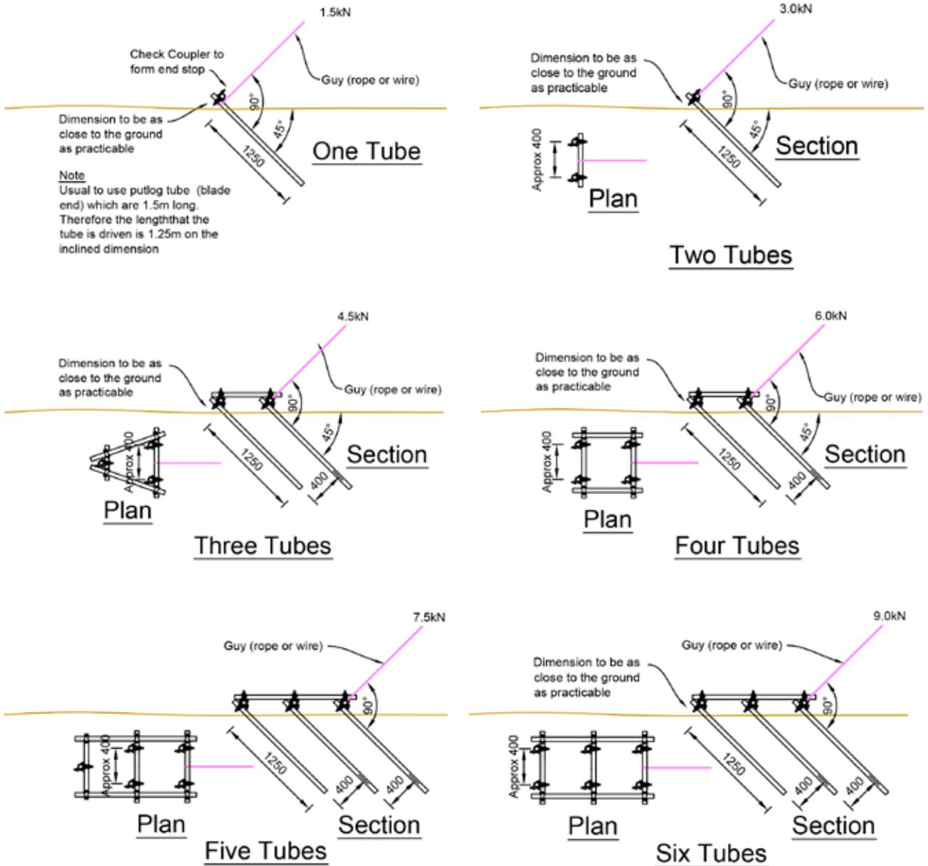
Figure 1 Tube Anchors
