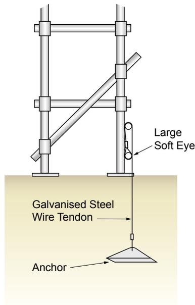
Figure 8 Method of Connection to Scaffold
