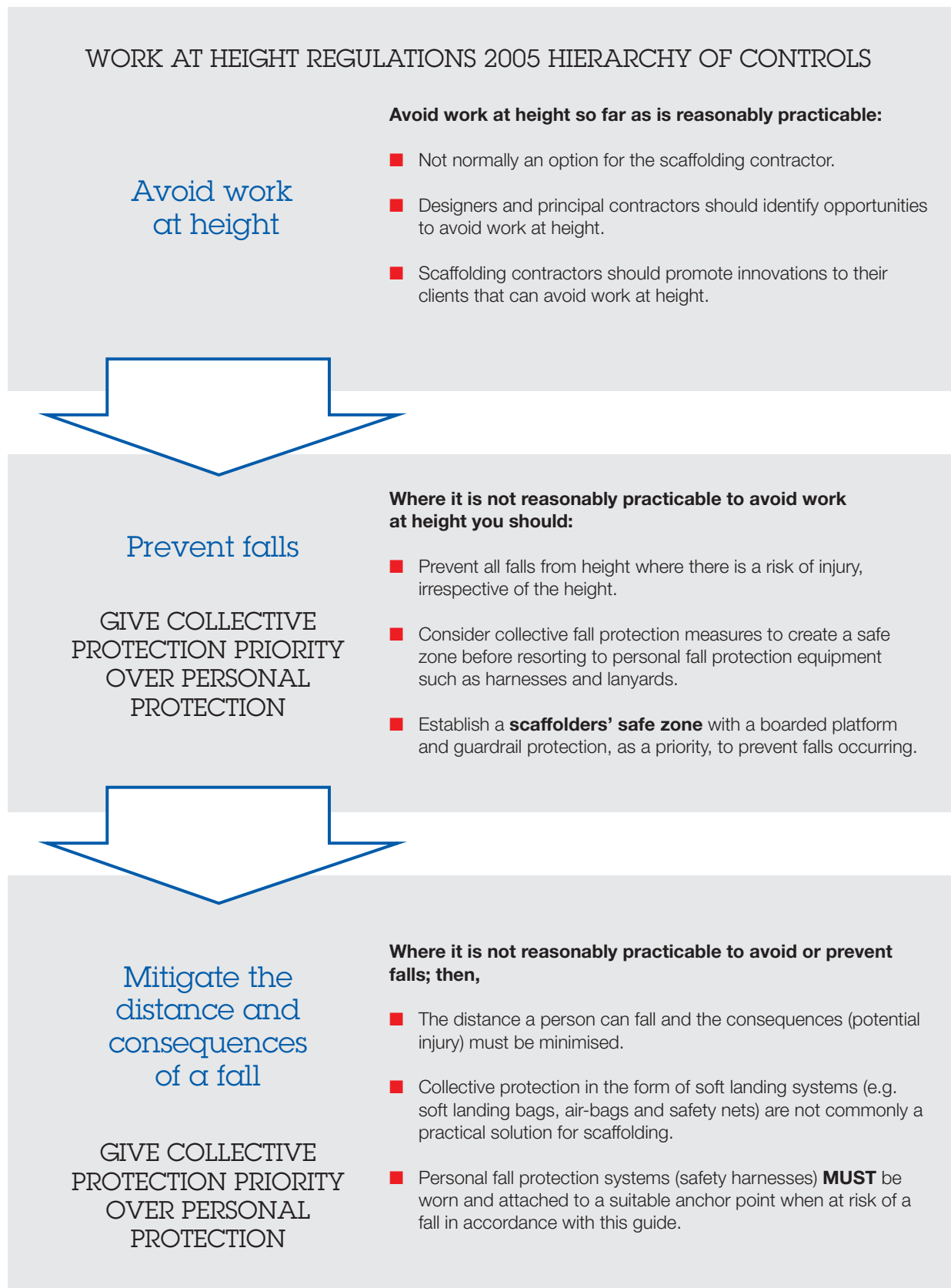
Figure 5: This diagram is a simple illustration of how the 'Work at Height Regulations 2005 Hierarchy of Controls' could be interpreted for scaffolding operations.
