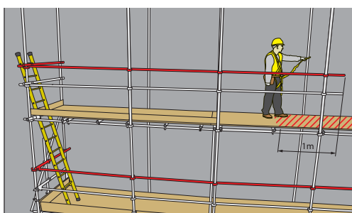
(iv) Attaching if encroaching within 1 metre of the end of the protected scaffolders' safe zone .
