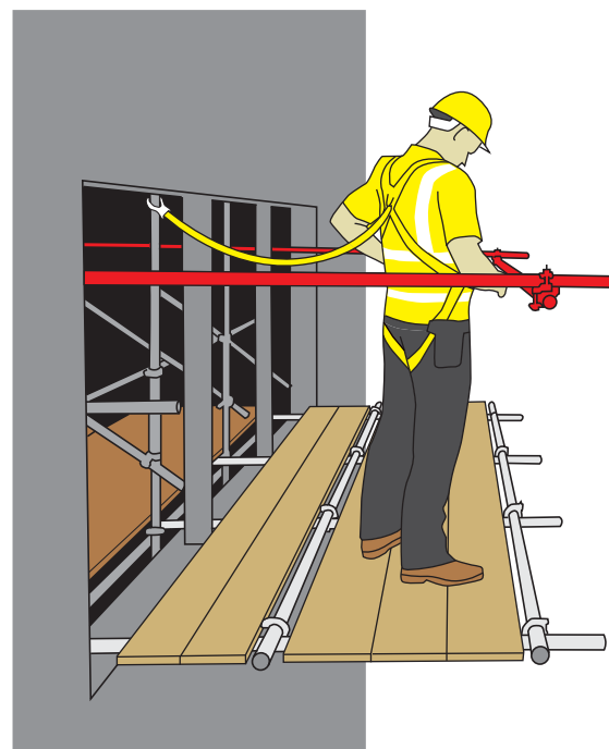
(iii) Needles are boarded out to create a scaffolders' safe zone to complete the truss-out scaffold.
