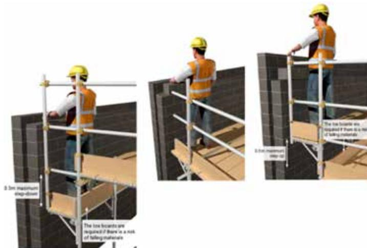
The platform may be fixed initially in the step-down position, then raised to the level of the main lift, and finally raised to the step-up position. This working method allows a scaffold with 2.0 m lifts to be used for bricklaying and blockwork, instead of a traditional bricklayer's scaffold with 1.35 – 1.5 m lift heights, allowing the scaffold to be used for other purposes without first adapting it to provide walkthrough lifts.
