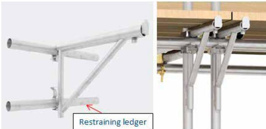
The inside platform should be level, with lapped boards only permitted at returns, and adjacent boards should be butted and supported. This requires a bracket to be fixed at each board end, plus at intermediate points to support the boards at their target spans.
