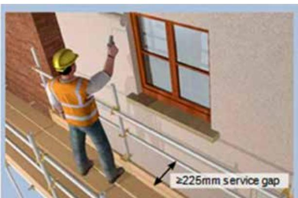
If the service gap exceeds 225 mm and a person could fall or suffer injury, double guard rails should be installed unless alternative arrangements are made to control the risk of falling personnel or materials as described earlier. Inner toe boards may be required for material retention subject to the risk assessment, although materials should not usually be stacked at the inner face.
