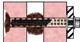
Resin stud anchors set in perforated brick using mesh sleeve to control the resin.
