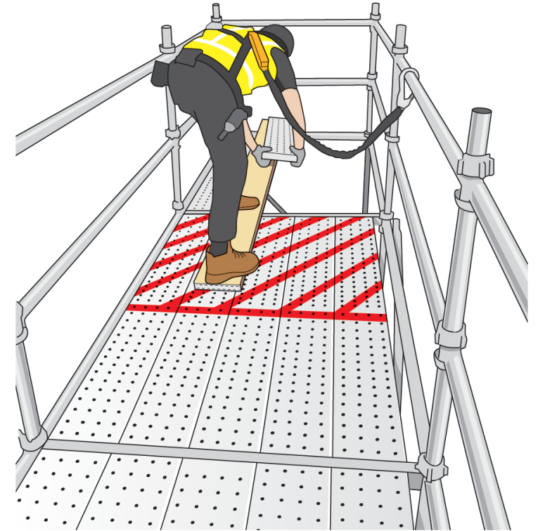
Example of an assembly aid to place and remove decking.
