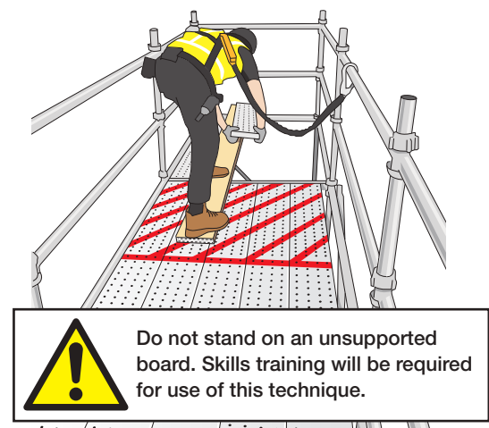
Figure 22: Example of an assembly aid to place and remove decking.
