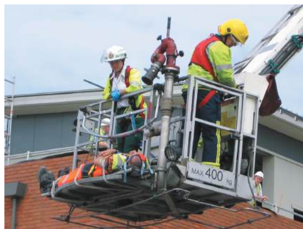
Figure 60: Recovery from height by emergency services. Shows the emergency services using a MEWP to recover an accident casualty from height.
