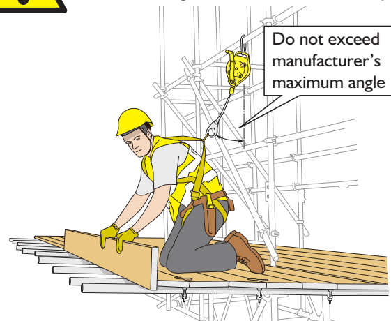
Figure 82: Falling object protection fan erected using a retrieveable inertia reel.
