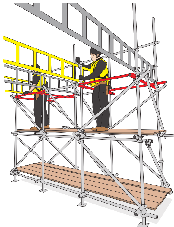
Figure 81: Examples of collective protection for the construction of gantry scaffolding.
