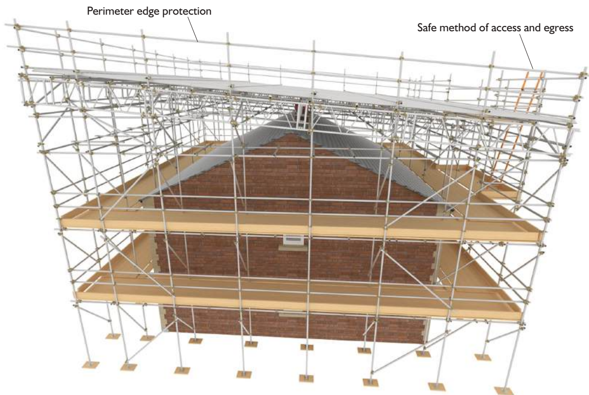
Figure 85: A traditional temporary roof incorporating edge protection and safe access and egress.
