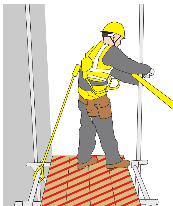
Figure 13: Example of Personal Fall Protection.
